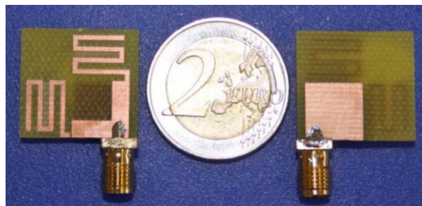
Figure 2.12: Pattern and polarization reconfigurable antenna[90]
