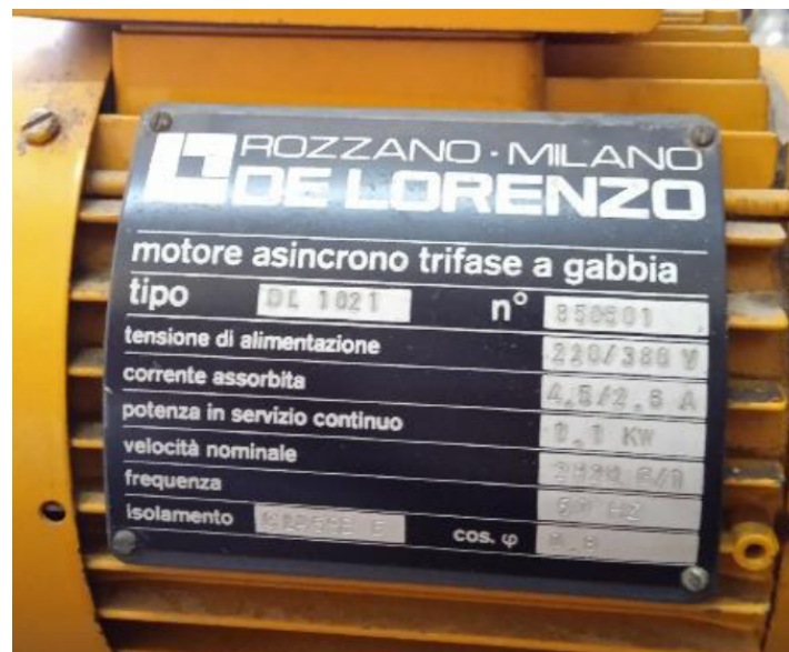
Figure 4.11: Induction motor nameplate
