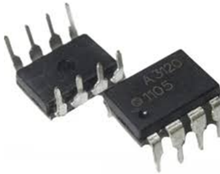
Figure 4.5: Integrated Optocoupler-Driver Circuit HCPL-3120
