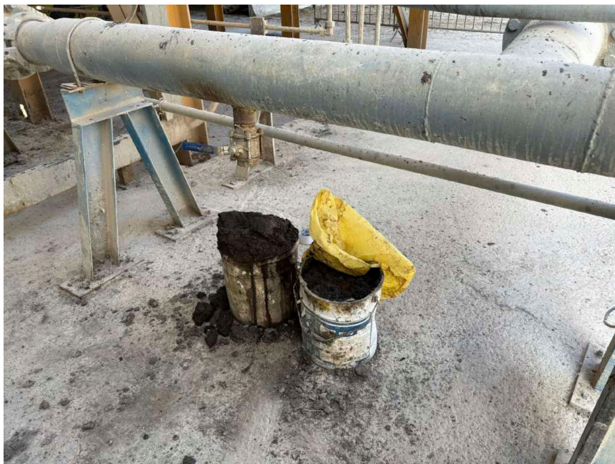
Figure 3.4. The alternative-fuel sampling station. At regular intervals a valve on the feed line opens and a grab sample is collected; the day's grabs are combined into a composite, a portion of which is analysed in the laboratory.
