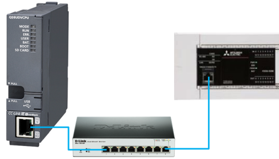
Figure 1.5: An example of PLC to PLC Ethernet Communication
