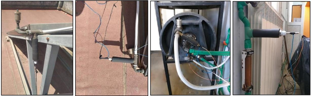
Figure III- 10: Positions of thermocouples on the different components.
