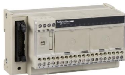
Figure 4. 9: Embase de raccordements.
