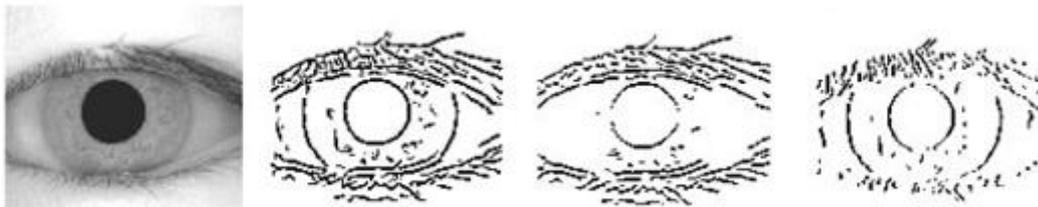
**Figure IV.8.** (a) Image initiale de *CASIA-Iris* (b) Image de contour diagonal
