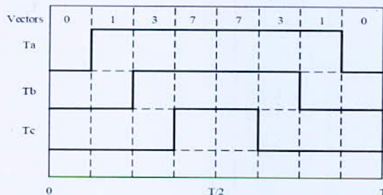
Fig. 2. SVM voltage vector timing
