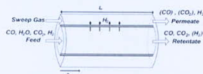
Fig. 1. Schematic representation of the membrane reactor
