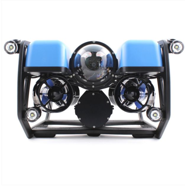
Figure 3.6: 4-Horizontal Thrusters Configuration
