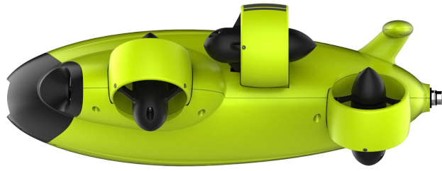
Figure 3.7: Vectored 6 Thrusters Configuration
