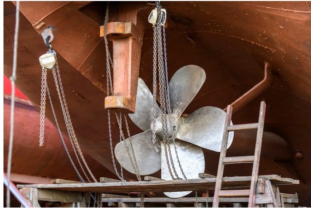
Figure 3.1: Fixed Pitch Propeller, from [2]
