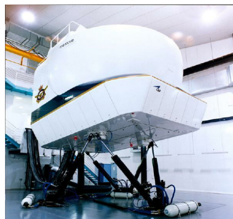
Figure 1.13: CAE flight simulator based on PKM by CAE Inc
