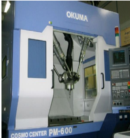
Figure 1.8: Cosmo Center PM-600: PKM-machine based tool by Okuma corp
