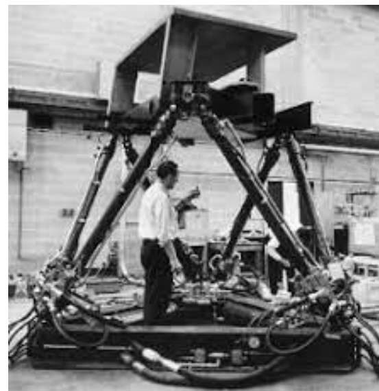
Figure 1.5: The first flight simulator based on a hexapod structure as in the mid of 1960s, from [16]
