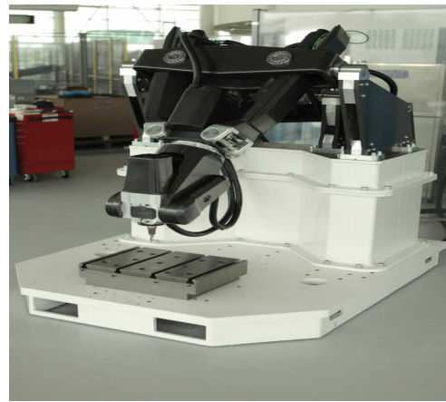
Figure 1.17: The Exechon robot: spatial manipulator with 3 exotic DOF by Exechon Enterprises LLC company
