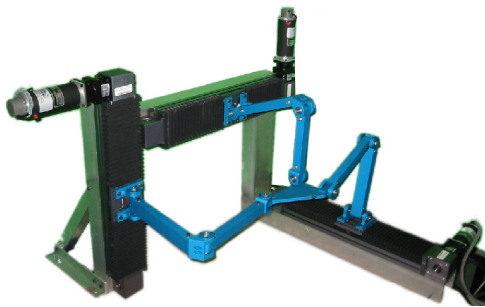
Figure 1.16: The Tripteron robot: spatial manipulator with 3 translational DOF developed by C.M Gosselin et al
