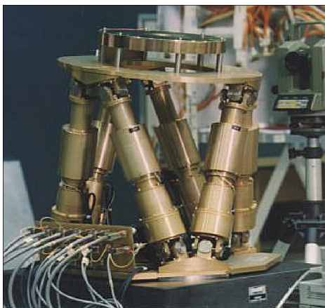
Figure 1.12: Hexapod PKM for satellite instrumentation by ADS International
