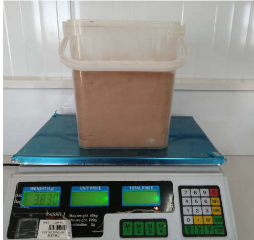
Figure 2.16: Weight of the soil after drying
