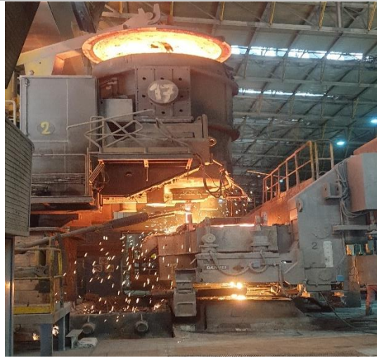
(a) The ladle is placed above the CCM; its content is unloaded in the tundish by gravitational forces
