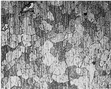
(d) Samples taken after a 1100°C, 3h heat treatment. Grains have nearly the same size as those of the previous treatment. Inclusions are nearly disappeared.
