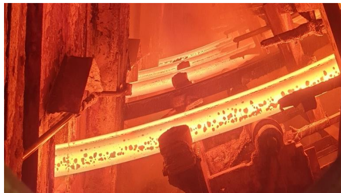
(b) The bending curve in the machine; billets have a soggy composition being solid in the interior and solid on the exterior
