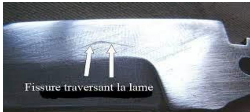
FIGURE I-14*: Cracks on a steel blade quenched but not tempered
