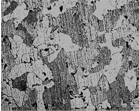
(b) Sample taken after an 800°C, 3h heat treatment. Bigger grains are observed (most of them still longitudinal, with some smaller grains between them). Inclusions density decreased slightly.
