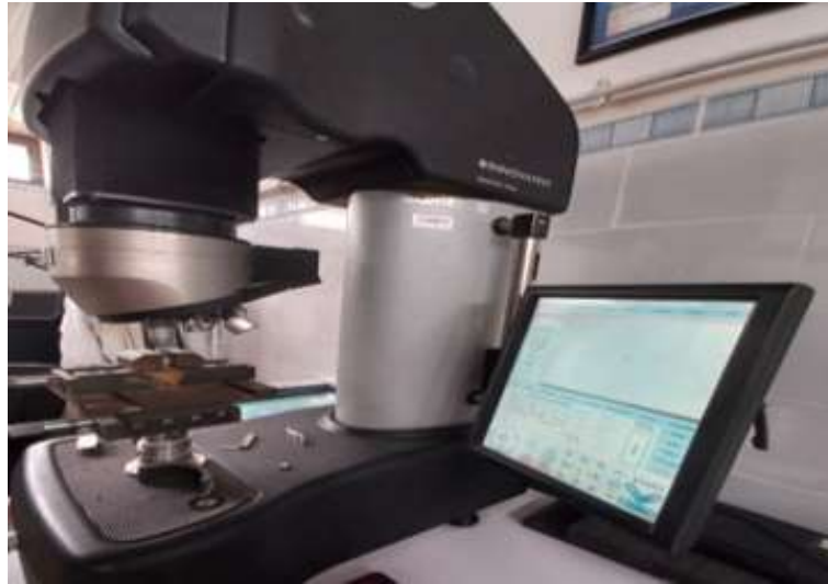
FIGURE 3.10 – Machine de dureté (INNOVATEST NEMESIS 9000)
