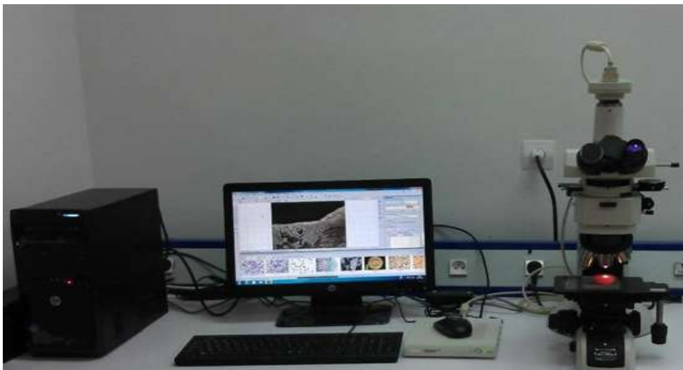
FIGURE 3.11 – Microscope optique (NIKON ECLIPSE LV100ND)
