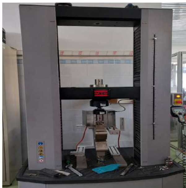
FIGURE 3.9 – Machine de traction (MTS Criterion model 45, 100 kN)
