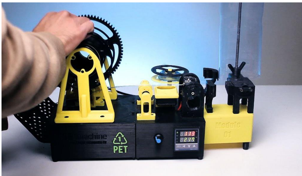
Figure 27: Cutting the bottle using gear motor
