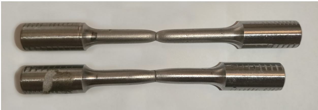
Figure 5.9: Comparison of plastic deformation between specimens. The base metal specimen is on top and the welded specimen is on the bottom
