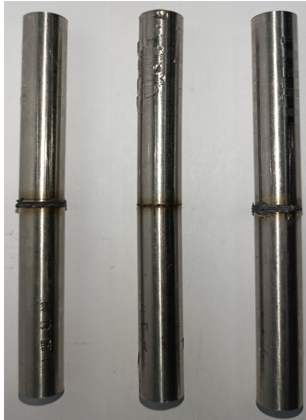
Figure 4.4: Failed welding operations
