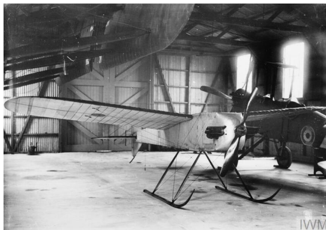
Figure 2.2: The Aerial Target, a British radio-controlled aircraft from the First World War.[6]
