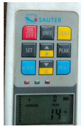
(b) Peak force result for the first model
