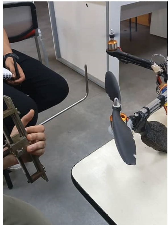
Figure 4.4: The experiment was conducted in FABLAB using the LGMD's Pitot Tube
