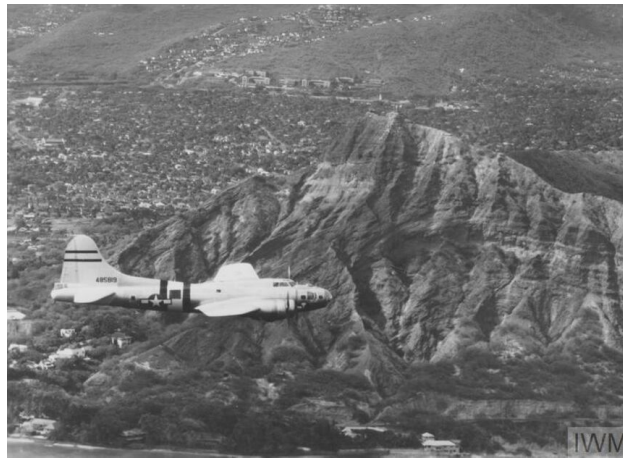
Figure 2.4: A remote-controlled drone prototype based on a B-17 Flying Fortress airframe takes off from Hilo Naval Air Station in Hawaii on 6 August 1946.[6]
