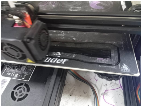
(a) 3D printing using Creality Ender3
