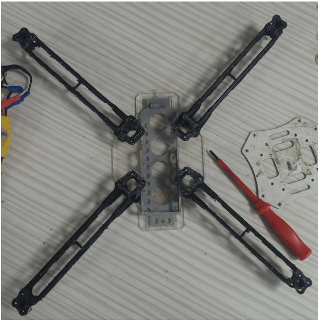
(a) Mounting the arms with lower base
