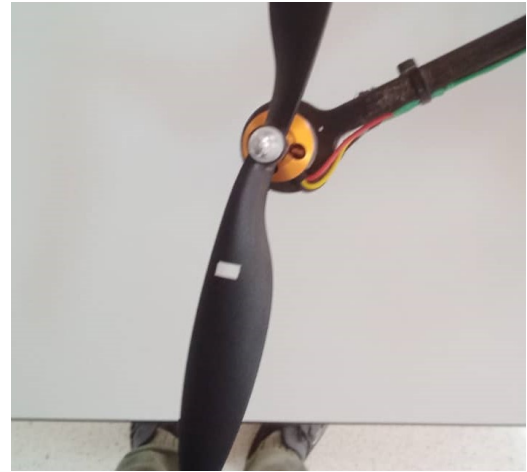
(b) Reflective tape added to one side of the propeller for measuring rotational speed
