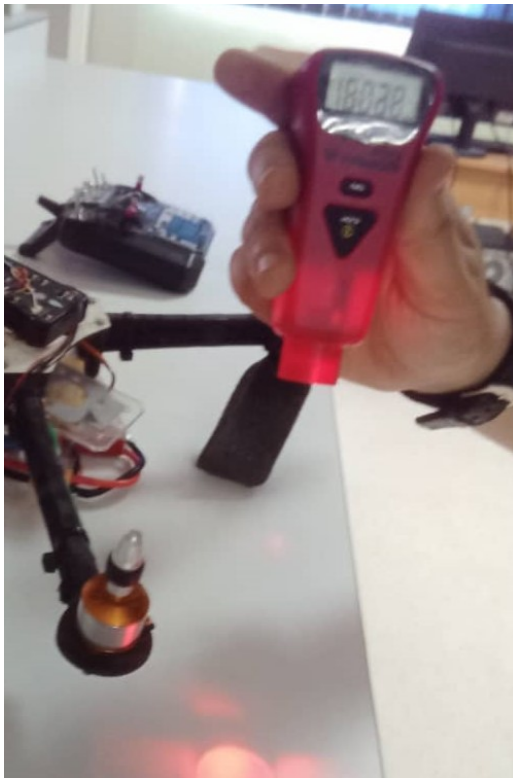
(a) Motor speed measurement setup
