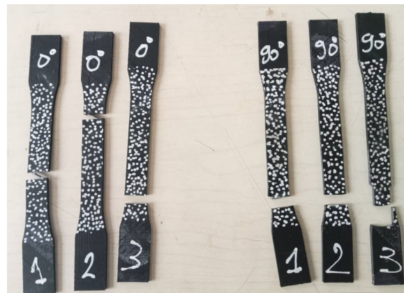
(c) Specimen after fracture
