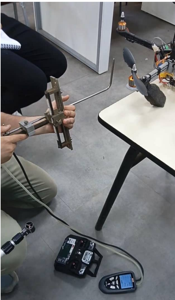
Figure 4.4: The experiment was conducted in FABLAB using the LGMD's Pitot Tube
