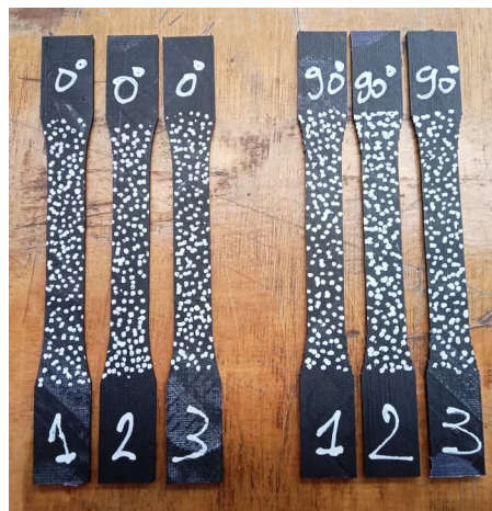
(c) Specimens after numbering and labeling
