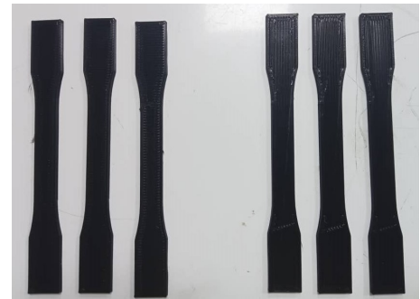
(b) Specimens after printing
