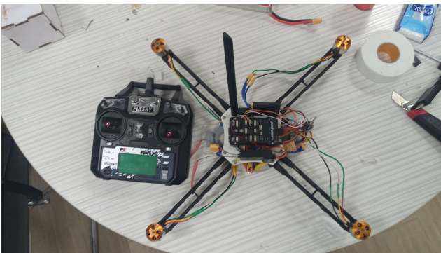
(c) Mounting the RC and Telemetry modules with flight controller
