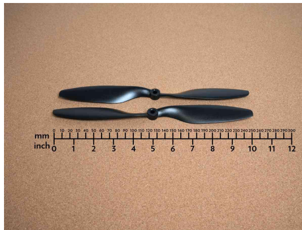
Figure 3.2: 1045 Propellers, one clockwise (CW) and one counterclockwise (CCW) to balance the rotational forces.
