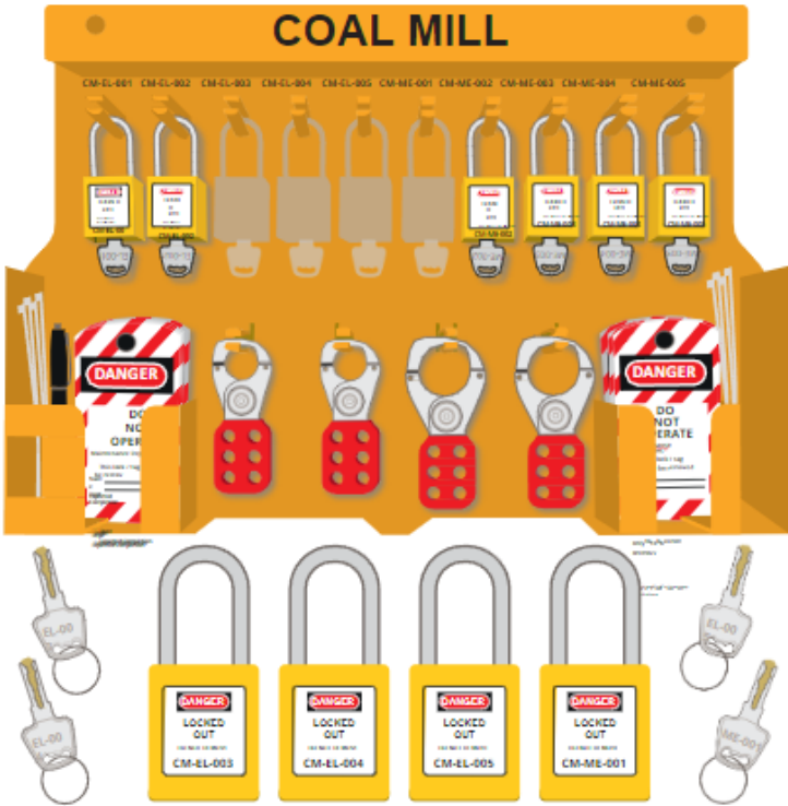
Figure A.1: Lock-Out Station
