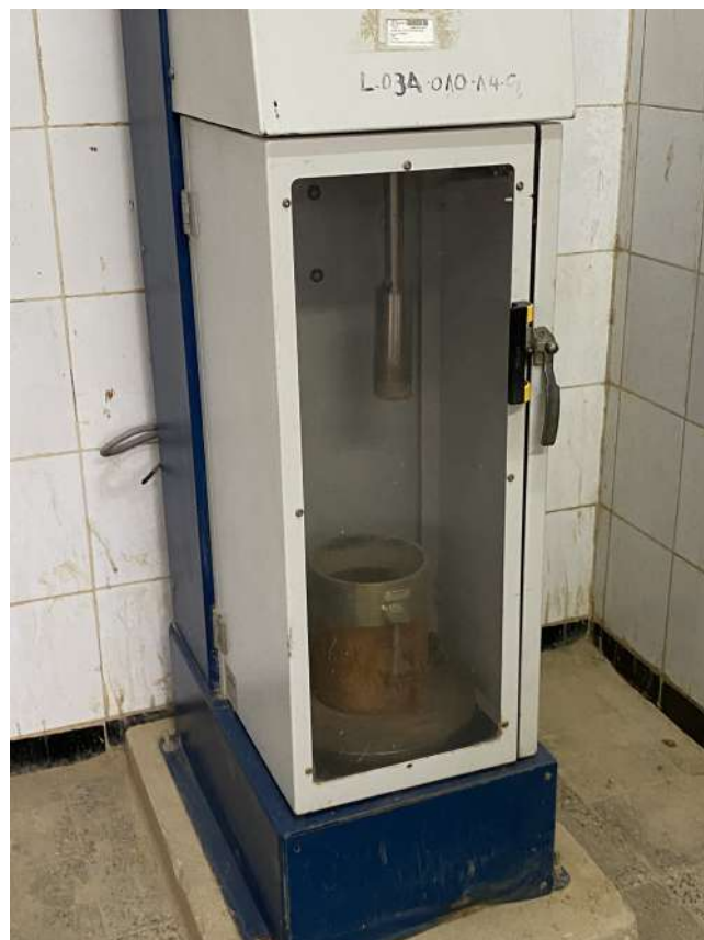
FIGURE 2.7 – Dame Proctor automatique
