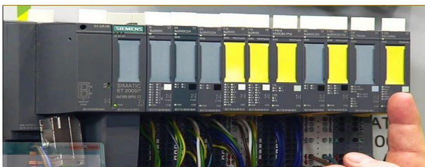
Figure 1.1 Automate programmable SIEMENS
