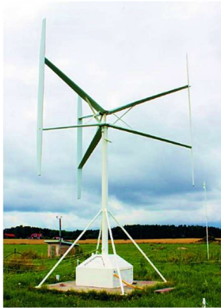
(a) 12 kW VAWT at Uppsala University 1 , Sweden rotor diameter: 6 m, hub height: 6 m, rated power: 12 kW (at 12m/s).
