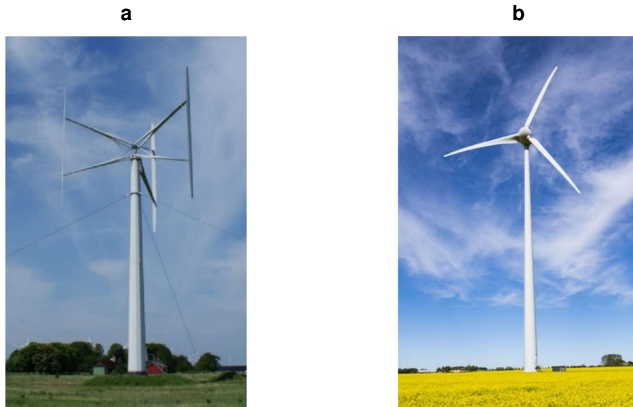
Figure 1: Wind Turbines: (a) Vertical Axis Wind Turbine [4], (b) Horizontal Axis Wind Turbine.
