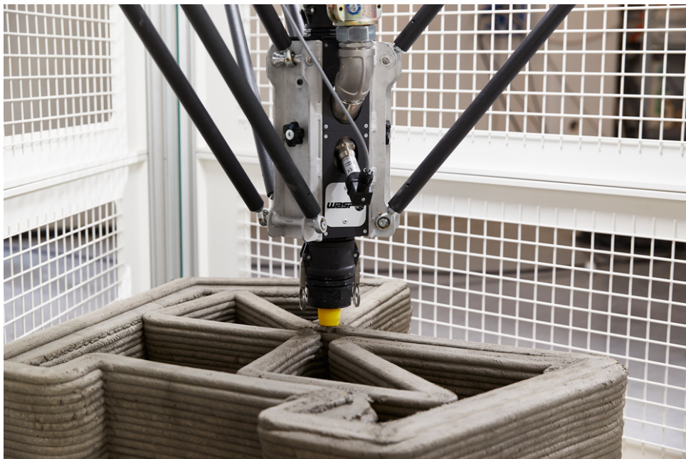
Figure 1.10: Delta WASP 3MT CONCRETE: Industrial-Scale Delta 3D Printer for Construction.
