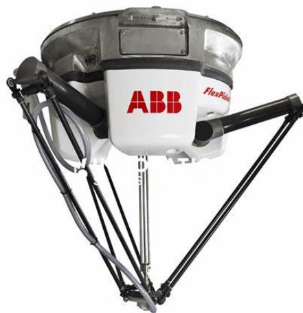
Figure 1.1: Modern Delta robot in a high-speed pick-and-place application.
