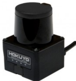
Figure 5.4: Hokuyo UST-05LA 2D LiDAR sensor
