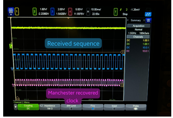
(b) Zoomed view of the received bit sequence and recovered clock
