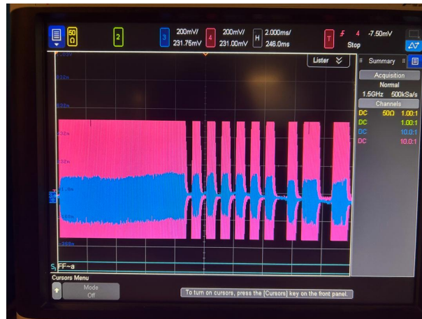
Figure 3.5: Effect of coil misalignment on received signal strength
