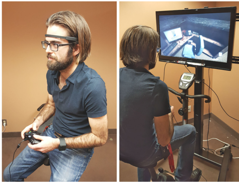
Figure 3.2: Experimental setup from the front (left). Experimental setup from the back (right). BioHarness 3 not shown since worn under the shirt.[41]
