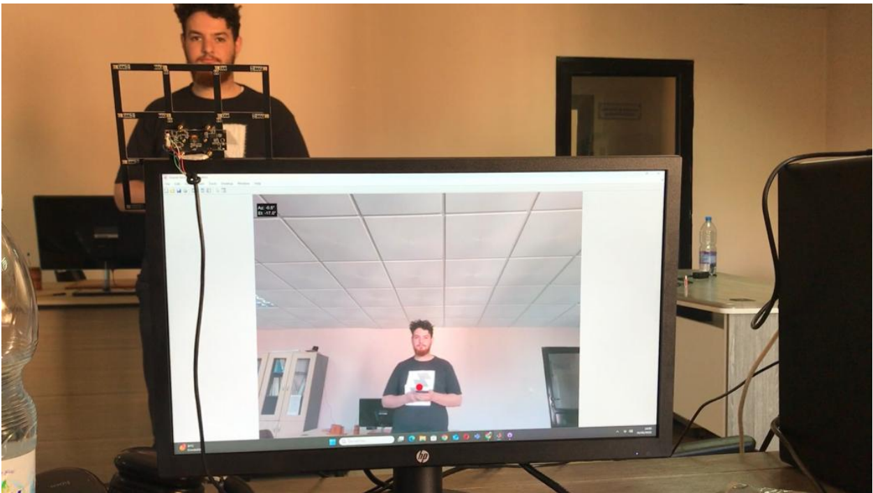
Figure 5.10: Example frame showing the DoA marker projected onto the live video stream without depth correction. The source is assumed to lie on a fixed unit sphere around the array.
