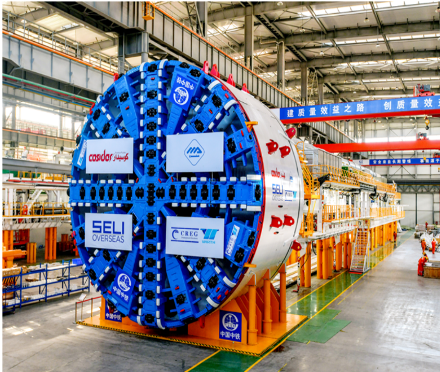
Figure 1.4: TBM “CREC665” Also known as KAHINA used for this project [6].
