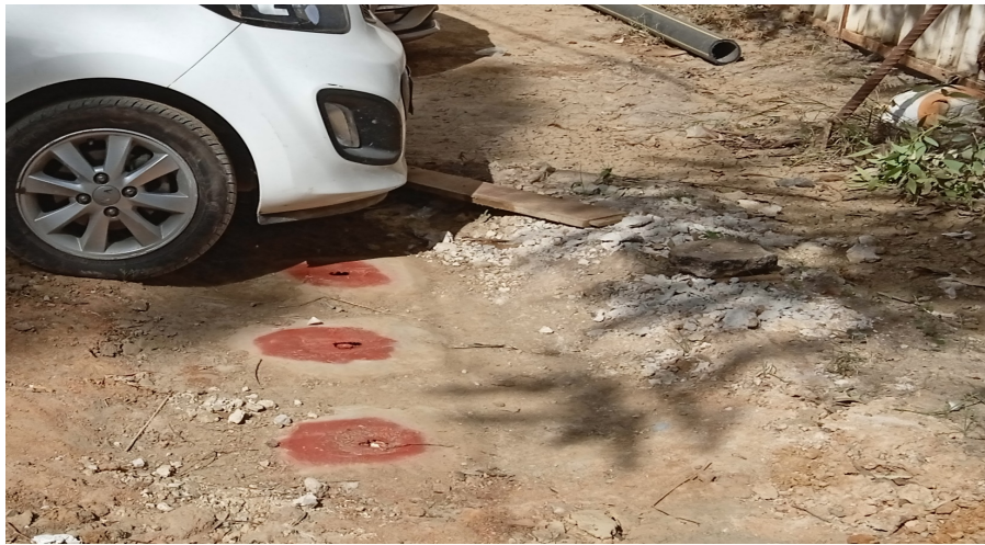
Figure 2.17: An array of settlement meters above the tunnel axis at pk2+654,00.
