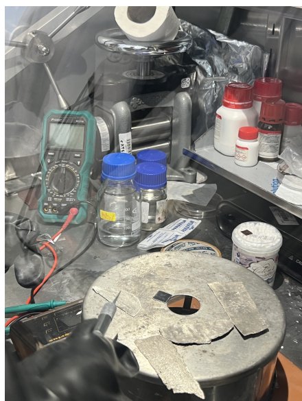
Figure 3.5 – Surface cleaning of lithium by gentle scraping to remove oxide layers.
