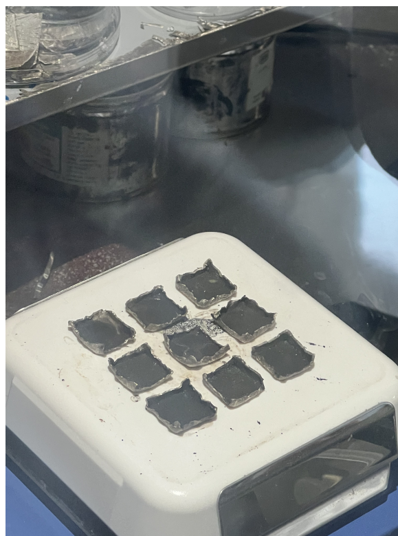
Figure 3.8 – Treated lithium surface after complete solution deposition.
