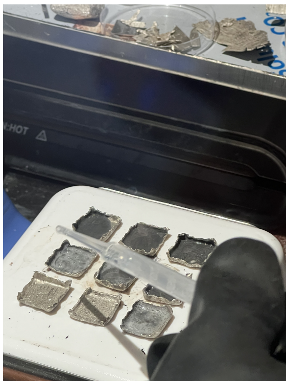
Figure 3.7 – Droplets of functional solution being applied onto the lithium surface.
