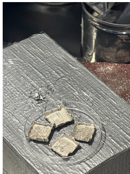
Figure 3.6 – Pure Lithium electrode prepared with raised edges before electrolyte application.
