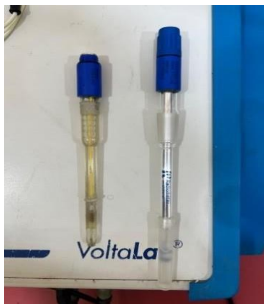
Figure 40: showing the Counter electrode, Reference electrode
