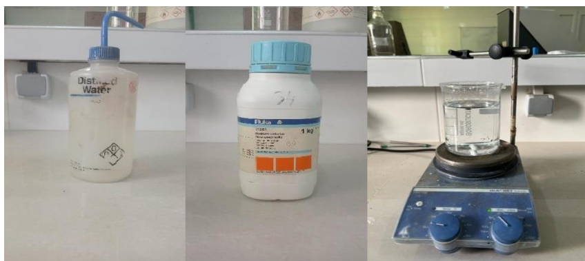
Figure 42: materials used for the preparation of 0.05M NaCl electrolyte (distilled water, chloride sodium and a magnetic agitator)
