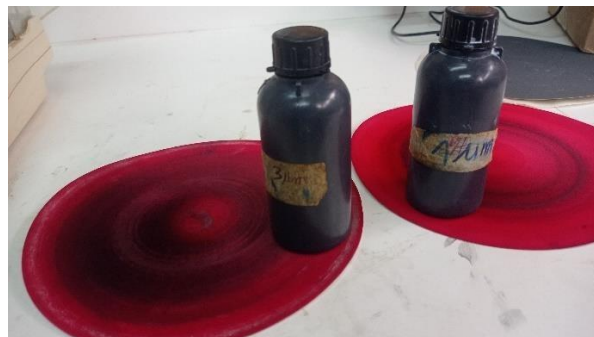
Figure 24: diamond paste suspension of 3 \mu m, then 1 \mu m.
