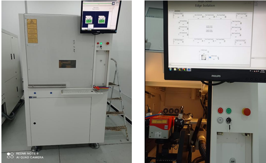
Figure IV.14 : ASYS SOLAR "Edge Isolation".
