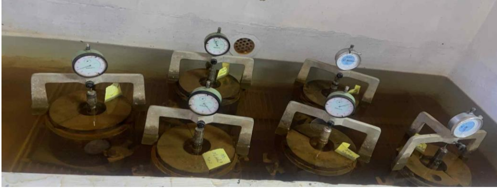
Figure 2.24: Immersion des moules CBR
