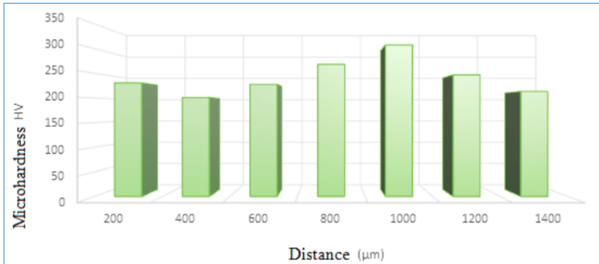
Figure 4.13: Microhardness profile of the spacer–cladding interface in Zircaloy-4 brazed with beryllium
