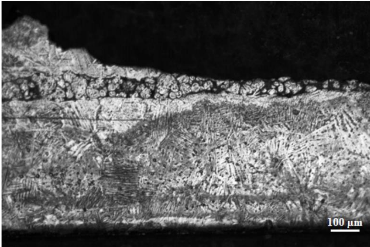
Figure 4.8: Excess beryllium defect in the brazing zone
