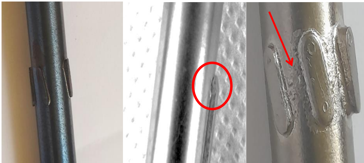
Figure 4.2: (a) Localized oxidation in the brazing zone, (b) Bonding defect, (c) Excessive beryllium at the joint
