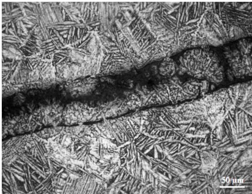
Figure 4.4: Microstructure of the brazed joint between the pad and the Zircaloy-4 cladding
