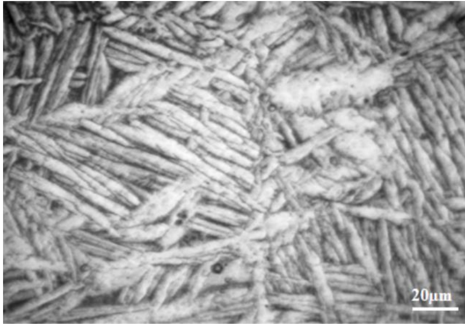
Figure 4.3: Microstructure of Zircaloy-4 cladding after brazing ( Widmanstätten structure)
