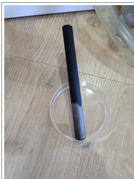
Figure 2.6: Manual spreading of the C/PANI paste on the graphite electrode
