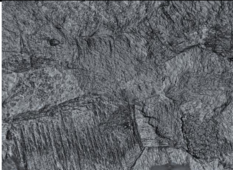
Figure IV. 5: Structures de Widmanstätten
