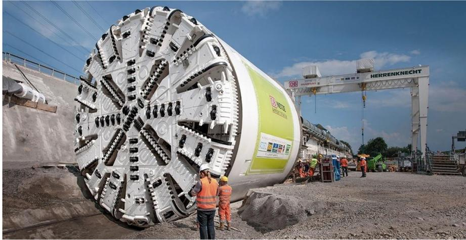
**Figure 1.5- Tunnelier TBM (Tunnel Boring Machine).(8)**
