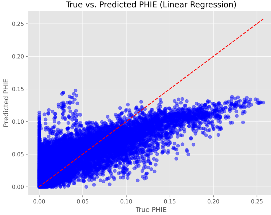
Figure 7.11: Measured vs Predicted PHIE for the test set using Linear Regression
