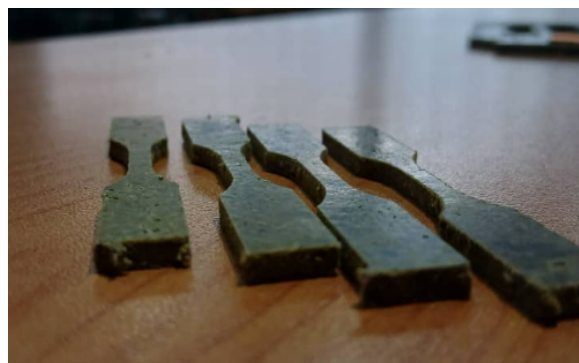
Figure 3.4: Tensile Specimens of 5% Fibers
