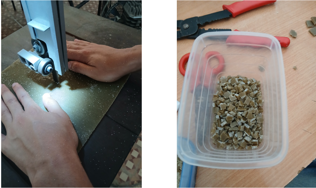
Figure 3.16: Pla/Palm Leaf Composite Pellets
