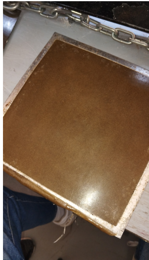
Figure 2.27: 300g Composite Material Plate
