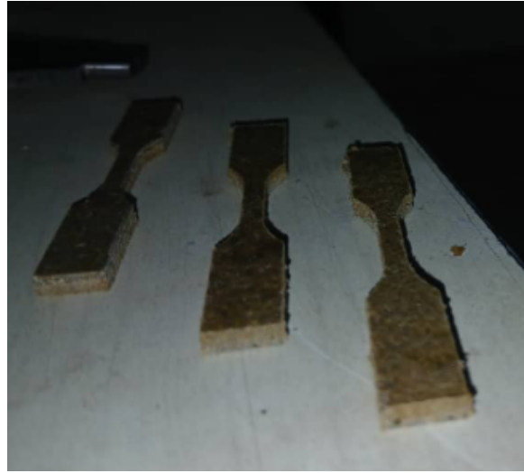
Figure 3.5: Tensile Specimens of 15% Fibers
