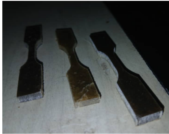
Figure 3.6: Tensile Specimens of 30% Fibers
