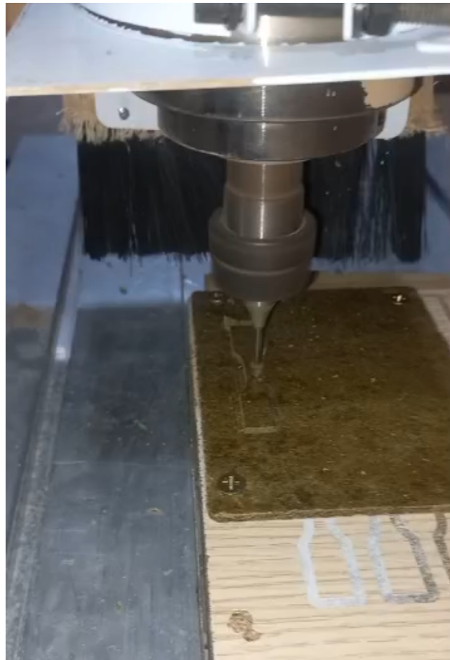
Figure 3.3: CNC Speciment Cutting
