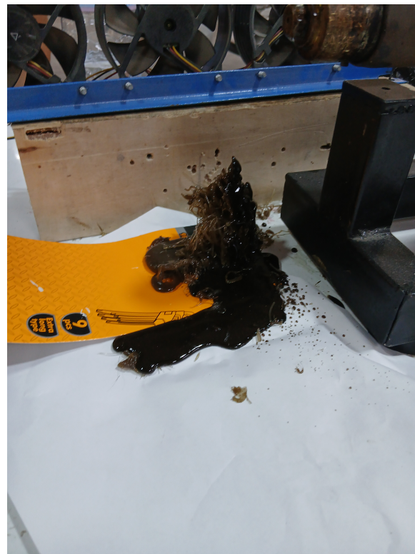
Figure 3.17: Failed Composite Filament Extrusion
