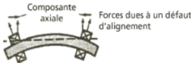
FIGURE 3.15 – Flexion du rotor
