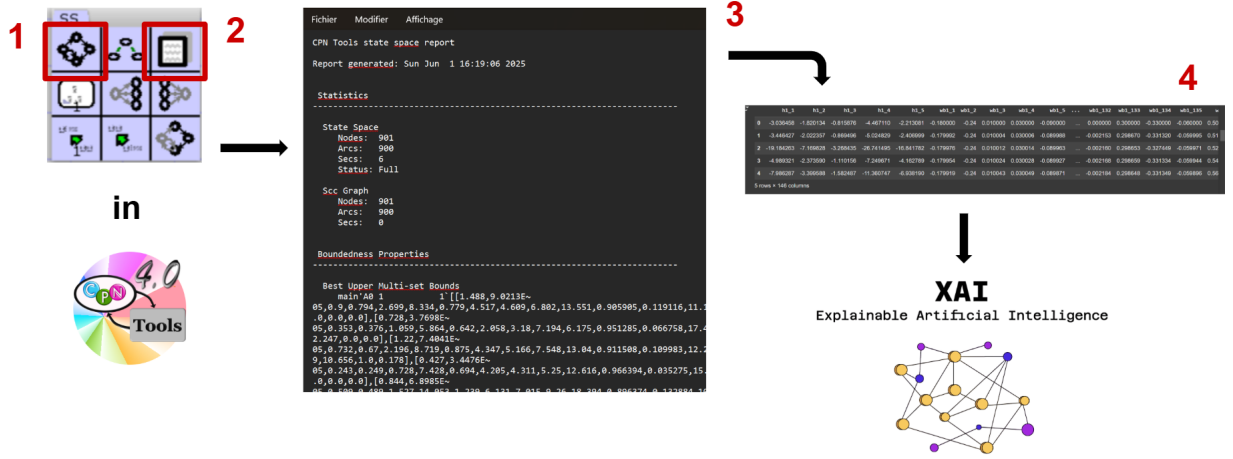
Figure 5.5: Pipeline for explainability via state space analysis in CPN Tools. (1) The state space and state space report tools are entered within the CPN Tools environment. (2) A full state space report is generated (3) Algorithm 1 extracts and structures the relevant numerical data into a tabular format. (4) This data is then used as input for Explainable Artificial Intelligence (XAI) methods to analyze and interpret the behavior of the modeled neural network.
