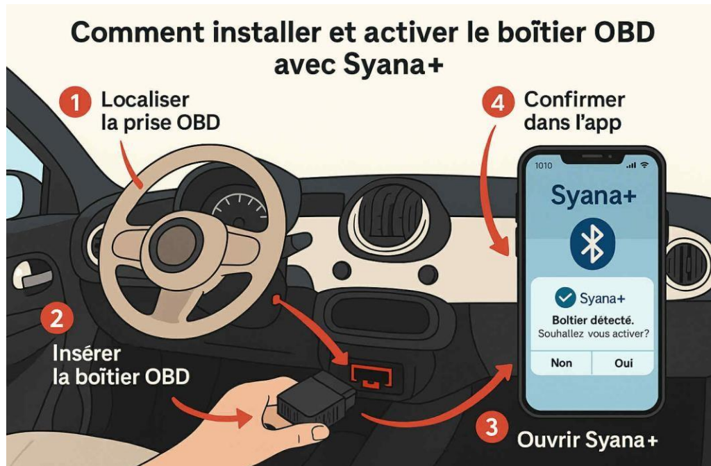
Figure IV.32: Installation et activation d'OBD
