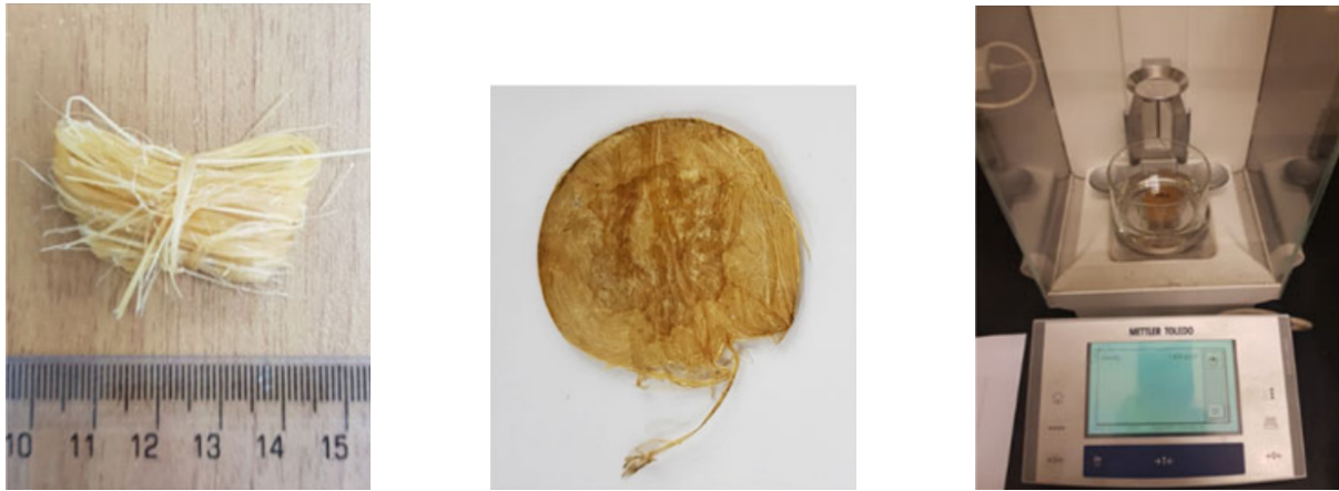
FIGURE 1.22 – Density samples preparation and measurement (adapted from Elseify et al. 2018)
