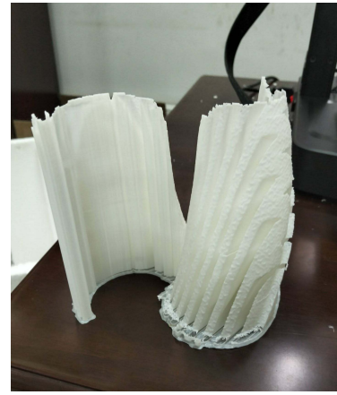
(b) Support structure used during printing
