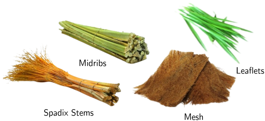
FIGURE 1.19 – Principal date palm fiber sources: spadix stems, leaflets, midribs, and mesh.
