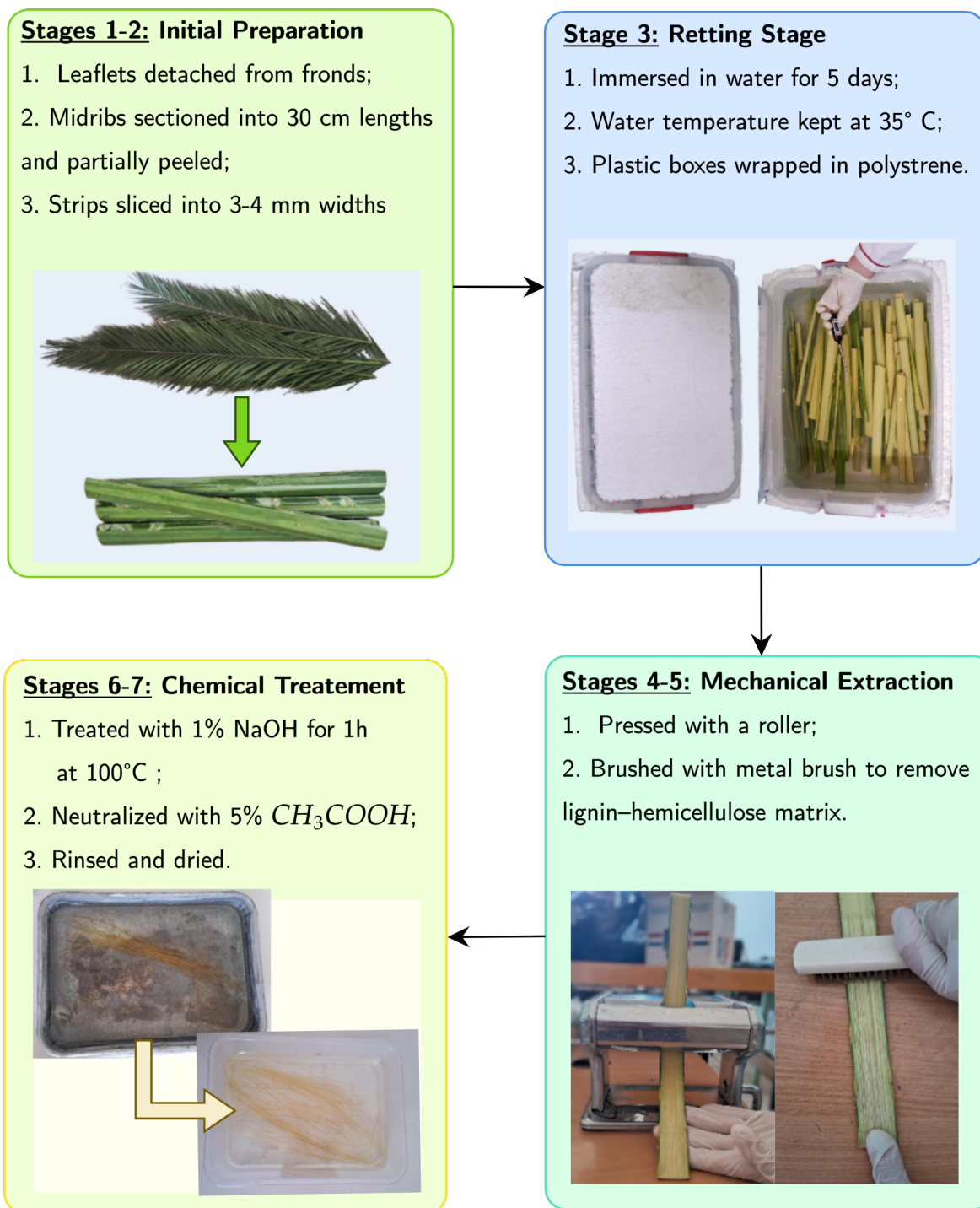
FIGURE 2.8 – Fiber Extraction from Date Palm Midribs (developed in this work)
