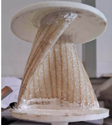
(a) Rotor bonded between upper and lower end plates.
