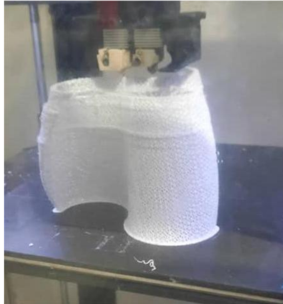
FIGURE 2.14 – Print improvement with reduced speed, but premature failure remains
