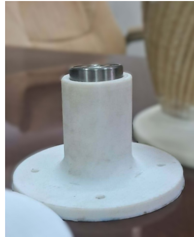
(b) Lower housing with bearing and spacer insertion.
