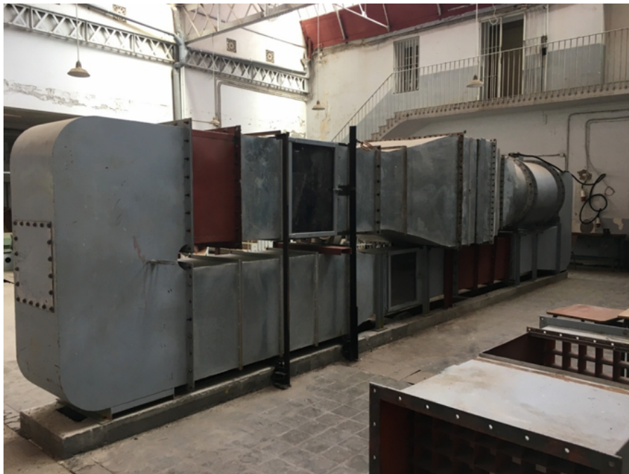
FIGURE 4.1 – Closed-circuit wind tunnel at the National Polytechnic School of Algiers. 1
