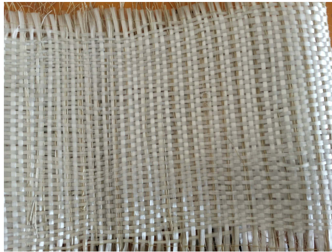
FIGURE 2.16 – Hybrid reinforcement fabric showing date palm fiber yarns integrated with fiberglass fabric
