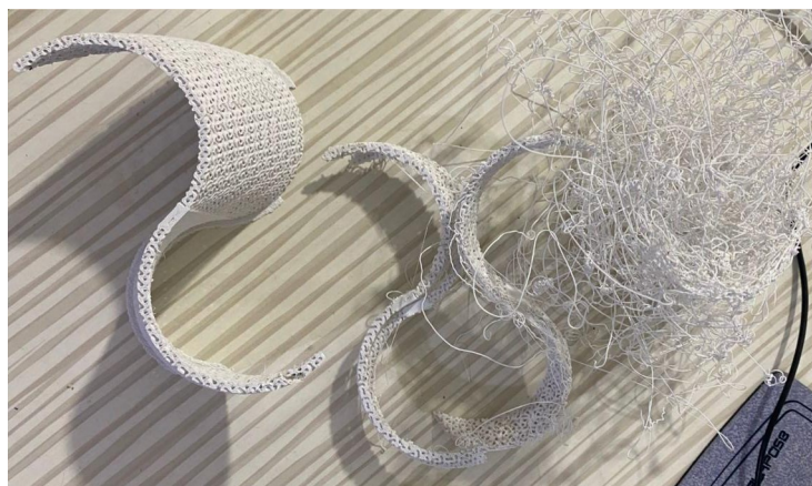
FIGURE 2.13 – Observed layer shifting at upper rotor heights
