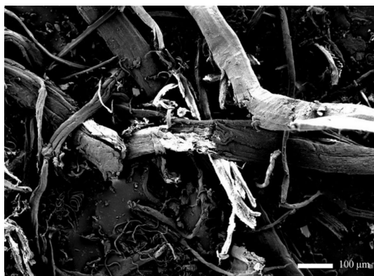
(a) Raw maguey fiber sample observed using SEM
