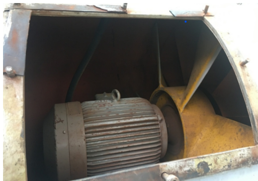
FIGURE 4.4 – Electric motor and axial fan assembly (adapted from [18]).
