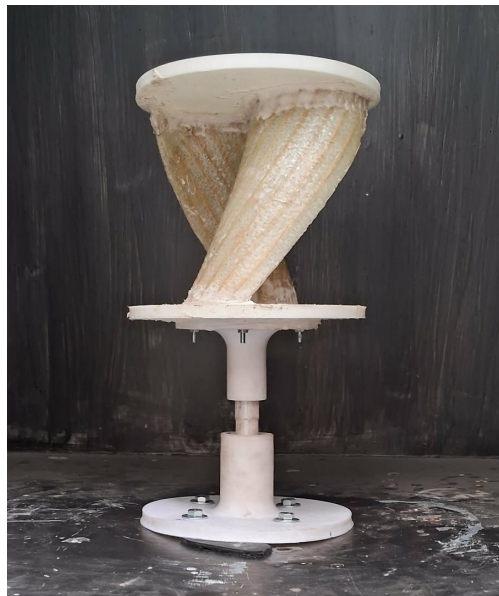
(c) Final assembled hybrid Savonius rotor.
