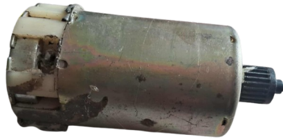
FIGURE 4.11 – Bicycle dynamo (3 W) selected for power generation
