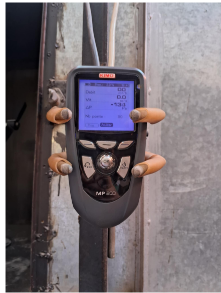
FIGURE 4.8 – KIMO MP200 digital manometer.
