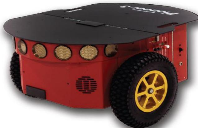
**Figure 4-5 : Robot mobil Pioneer 3-dx**
