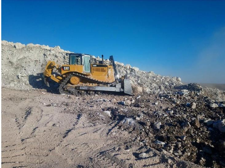
Figure III-4: Bulldozer Caterpillar D8R
