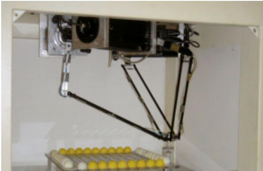
Figure I.3 – Robot Delta de l'EPFL [1]
