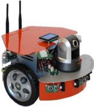
Figure 1.7 :robot mobile (Version Pro) WiFi X80SVP Dr. Robot source [4 int]
