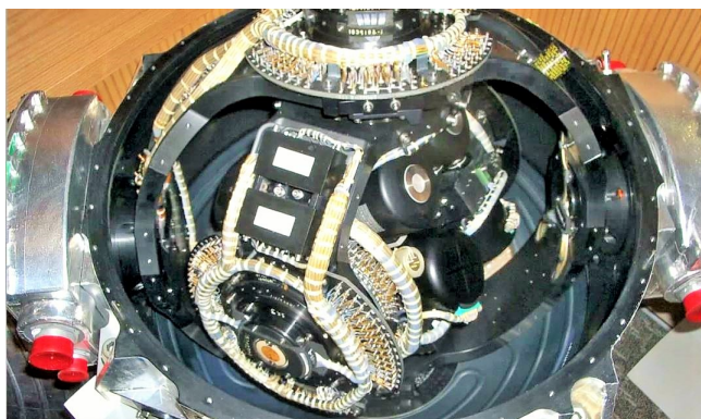
Figure 1.1: Example of early gimballed inertial systems used in missiles [2]
