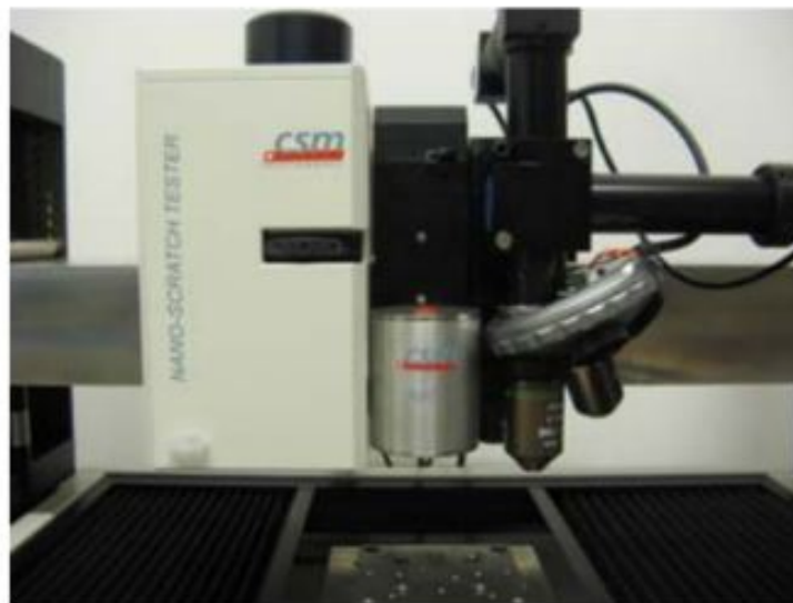
FIGURE 4.7 – Nanoindentation tester (NHT) de CSM. Source : [35]
