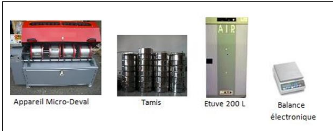
Figure II.6. Appareillage de l'essai Micro-Deval [17].
