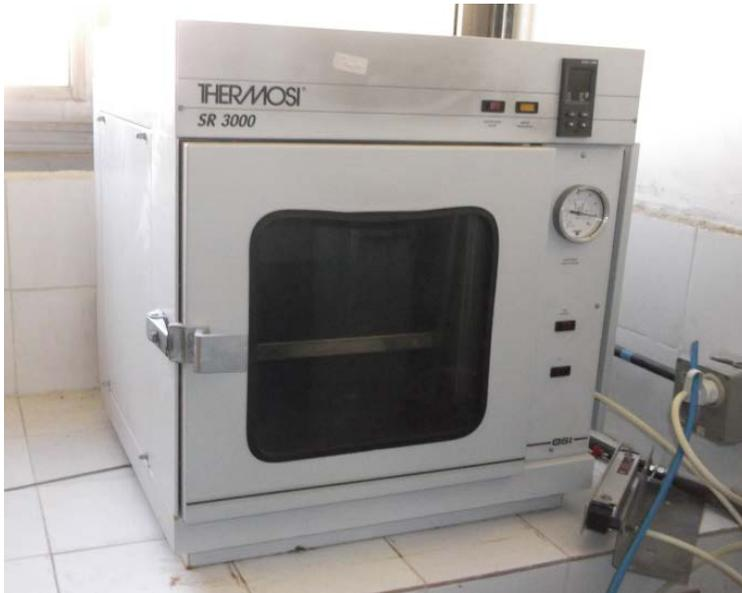
**Figure III.4** : Etuve de type THERMOSI SR 300.
