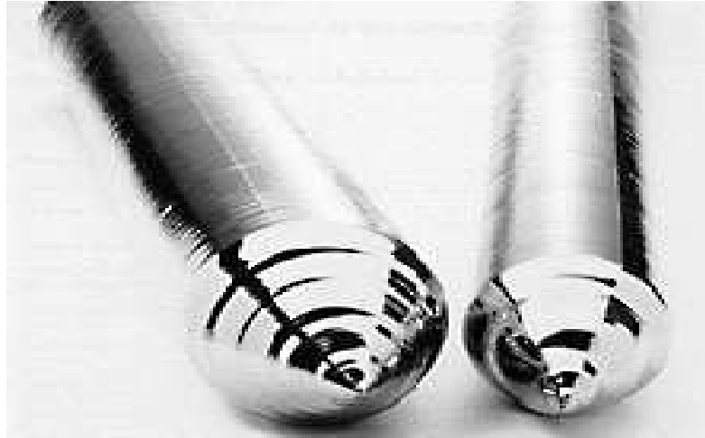
Figure I.25: Lingots de silicium monocristallin [28].
