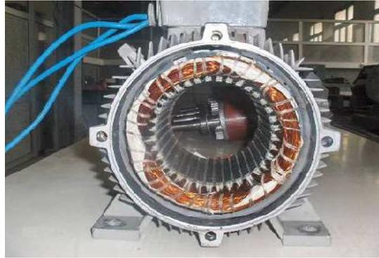
**Figure (B-2):** stator de la machine asynchrone.
